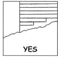
**FOUNDATIONS:** Visible foundation walls are limited to less than 18" vertically.
